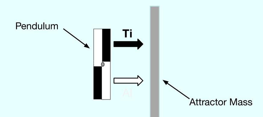
As the attractor mass is oscillated, any interaction dependent on the composition difference of the right half of the pendulum would result in a modulation of the twist, and could be evidence of a short-range violation of the WEP.
