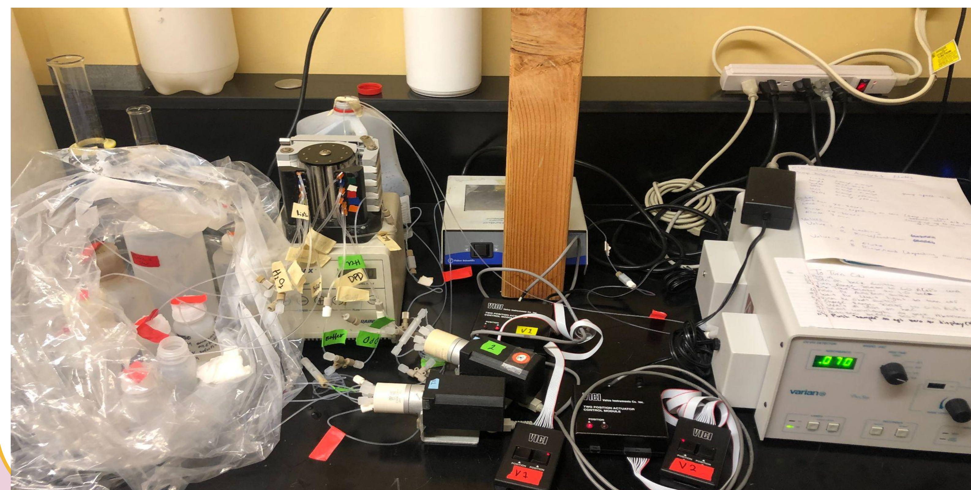
Figure 2. Peristaltic pump set up with temporary metal clean space, attached to a UV-Vis spectrophotometer.
